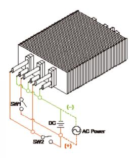
Power Switch Circuit Setup for Low, Medium, and High:
